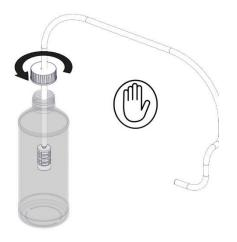
3. Open the chemical injector by turning the knob anti-clockwise until the desired affect is reached. When the trigger is pulled, water mixed with detergent will be sprayed.
